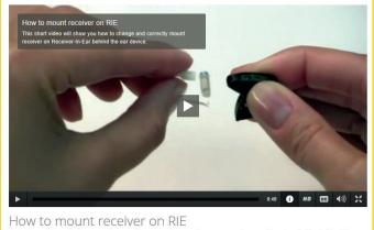
This short video will show you how to change and correctly mount receiver on Receiver-In-Ear behind the ear device.
